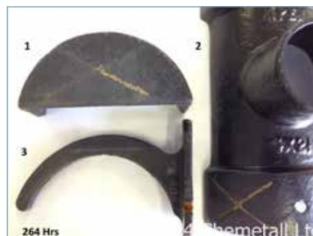
**Alumasc's certified factory painted finish at 264 hours of accelerated weather testing...**
